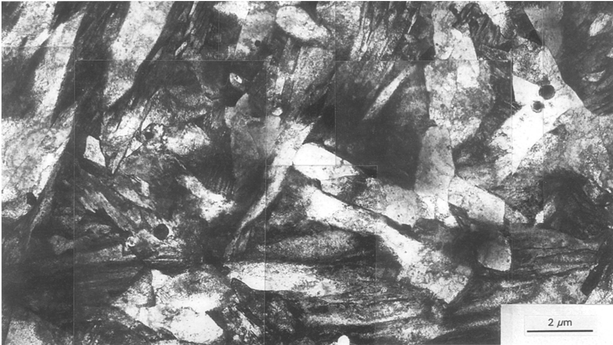
Figure 9 Transmission electron micrograph showing the microstructural details of the specimen with 15% deformation of austenite at 700 °C followed by isothermal transformation at 540 °C for 10 min.
